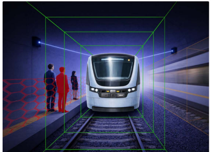
StandClear™ in operation — sensor fields detecting platform encroachment in real-time.
